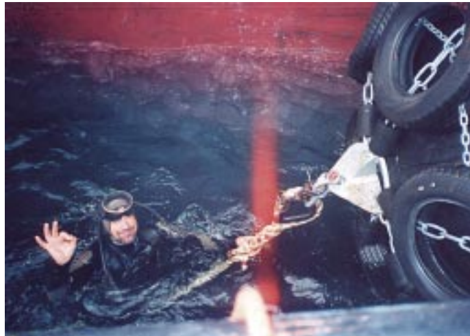
Fenders are lowered and set in place by divers in lightering operation from the Castor to the chartered tanker Yapi. Photo on facing page shows the Castor with the Nikolay Chiker in attendance.
