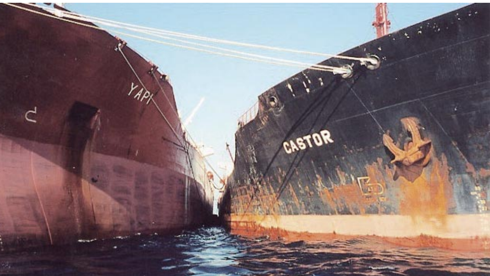
Fenders are lowered and set in place by divers in lightering operation from the Castor to the chartered tanker Yapi. Photo on facing page shows the Castor with the Nikolay Chiker in attendance.
