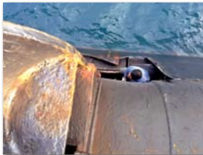
Significant weather deck damages / distortions required temporary repairs to restore the ship's hull integrity and mooring capability.
