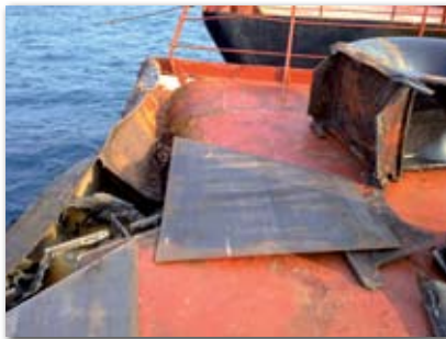
Significant weather deck damages / distortions required temporary repairs to restore the ship's hull integrity and mooring capability.
