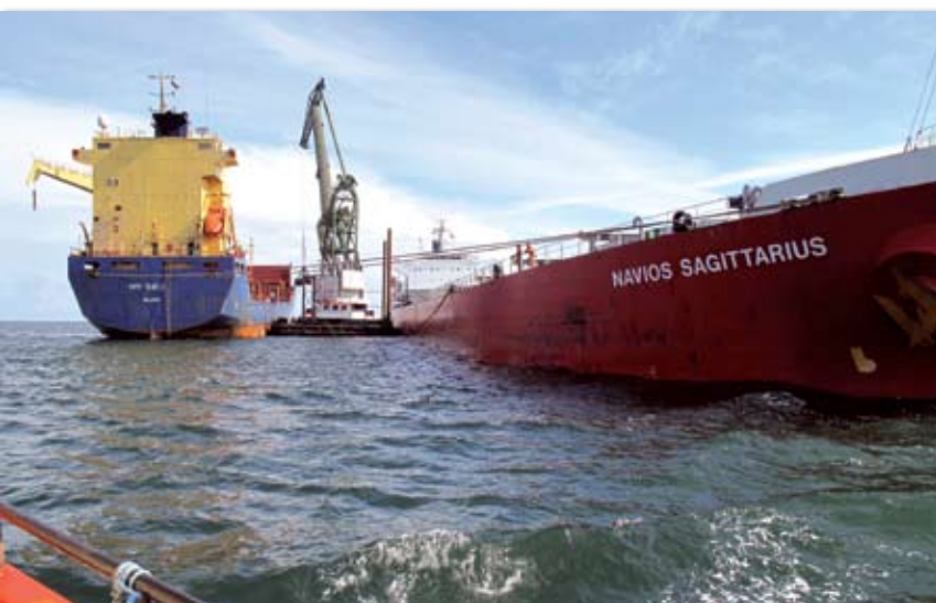
The casualty was successfully refloated following lightening of about 3,000mt of cargo
