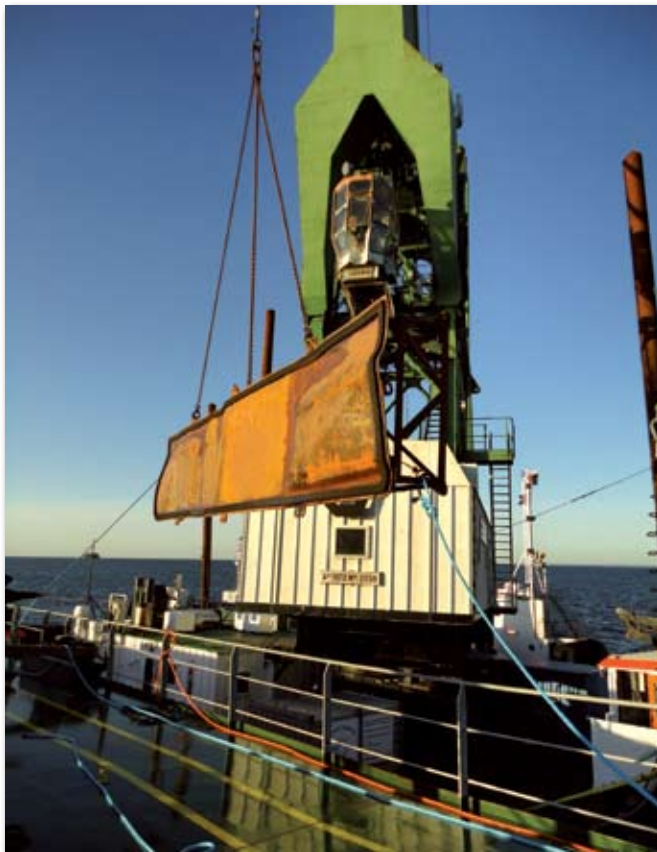
Doubler plate (8x2mtr) shaped to fit hull's actual deformation, was lowered into position, and welded by divers by way of the hull bottom rupture.
