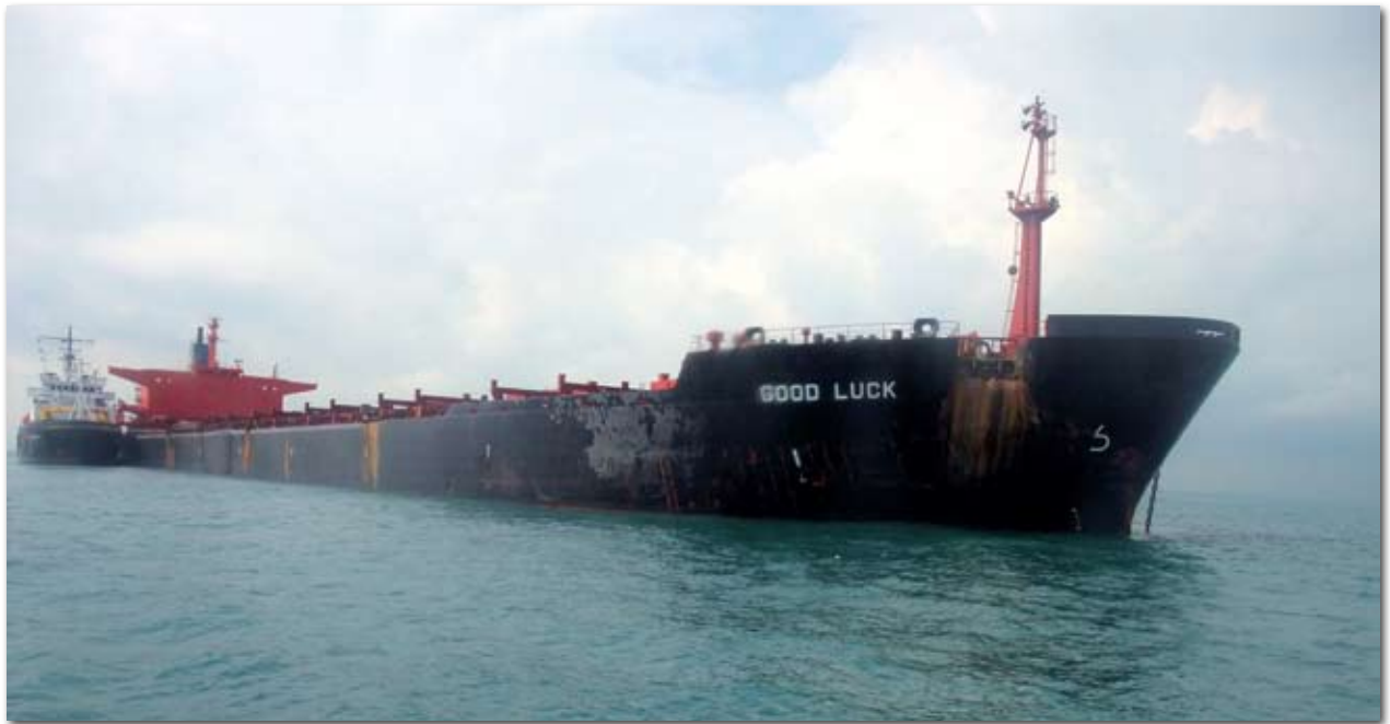
Capesize bulk carrier GOOD LUCK, 175,000dwt, laden with iron ore, lost both anchors and collided with numerous vessels anchored off Singapore, sustaining severe damages.
